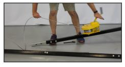
5. Align the upper beam with the jack frame piece; make sure that the cable is not twisted around the beams. If the jack is being assembled with the base plate downward, the kickstand will be on the right side of the beam looking from the wheels. Make sure the cable runs straight from the winch to the pulley at the top of the upper beam.
