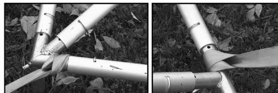
5. Fasten the loop strap (B) to the fitting at each leg location.
