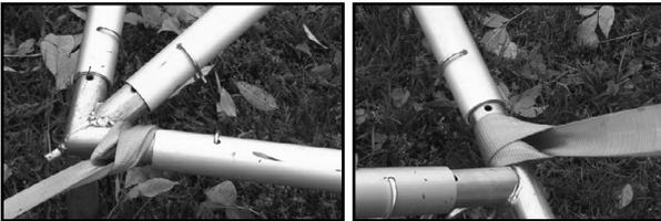
6. Roll out a drop cloth to protect the tent top of dirt and abrasions next to the frame and unroll the tent top pieces. The tent needs to be laid out in the sequence of: 20x10 lace end, 20x10 midsection, 20x10 grommet end. (The midsection has a lace and grommet side; each seam requires one lace line and one grommet line for fastening.)
