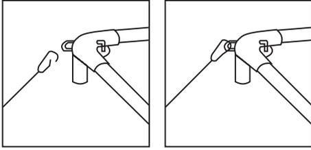
10. Place stakes 5' out from each leg; drive stakes into the ground so that approximately 6" or less of the stake is showing.
