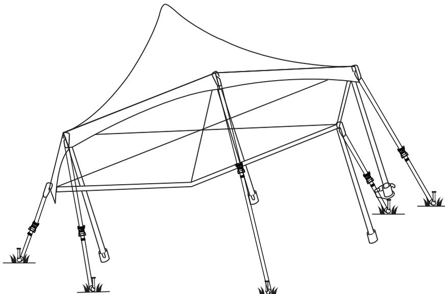
13. Fasten the 6' series loop strap (D) to each corner through the two metal O rings on the tent top, then through the end loop and tighten.
