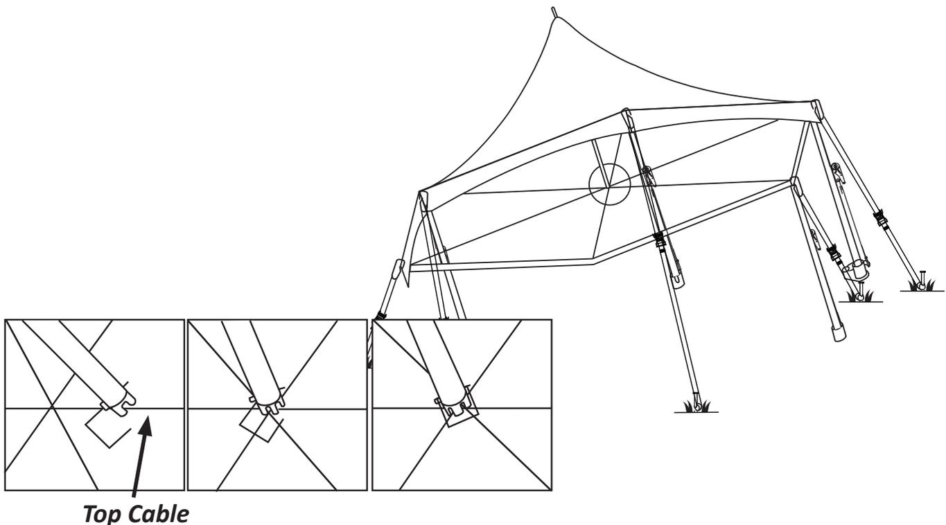
16. Install the remaining two legs (8') and ratchet assemblies; be sure the smaller holes of the base plate are facing the interior of the tent.
