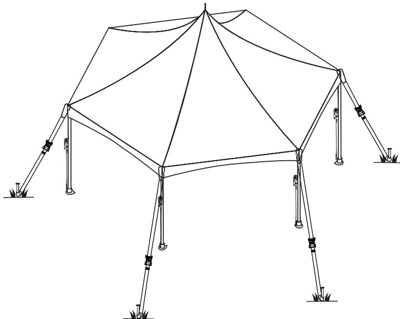
17. Make sure the legs are straight then secure each base plate by driving a 24" anchoring hooks into the smaller hole of the base plate tighten all ratchet assemblies.
