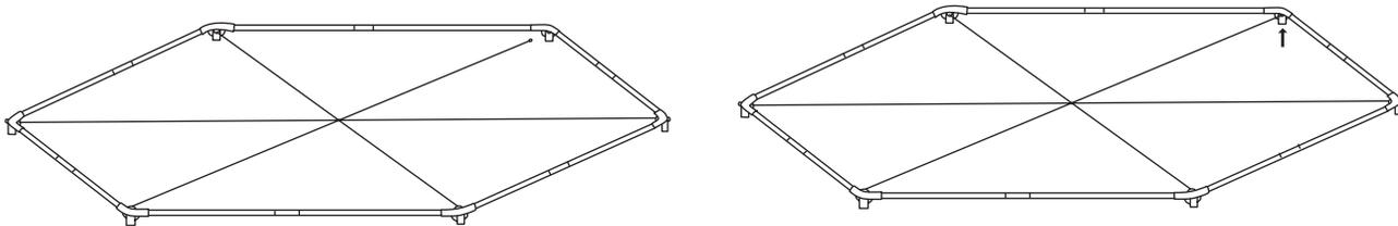
8. Lay the tent top out over the cables and frame with the top of the tent facing upward. Start in one corner by securing the white nylon strap over the ring on the outside of the corner fittings.
